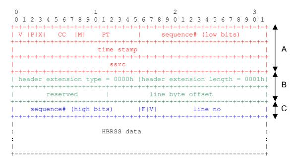
In the above diagram the red section A is the RTP (RFC3550) header, the green section B is the RTP header extension (formatted as specified in RFC3550), and the blue section C is the payload (RFC3497) header.
